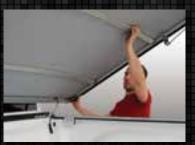
FAST AND EASY REMOVAL Gas shocks are designed to be easily removed by hand using a ball and joint snap release. No tools needed. Leave your tonneau at home within seconds.
