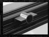
Spring-loaded bows rest in rail system and provide horizontal tarp tension. Bows conveniently roll-up within tarp when tonneau is not in use.
